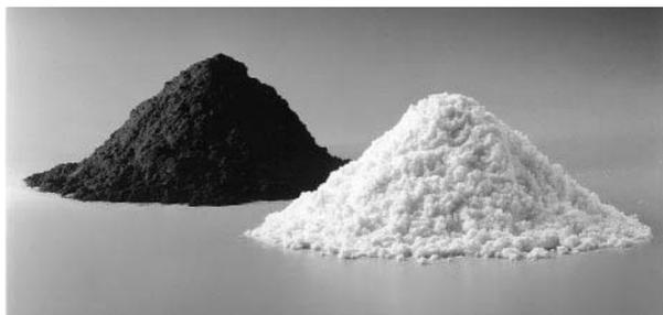
**Figure 1** Powdered ion exchange resins.
