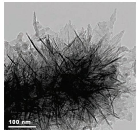
Figure 1: Nanoalumina fibres. Photograph by R.Ristau, IMS, UCONN
