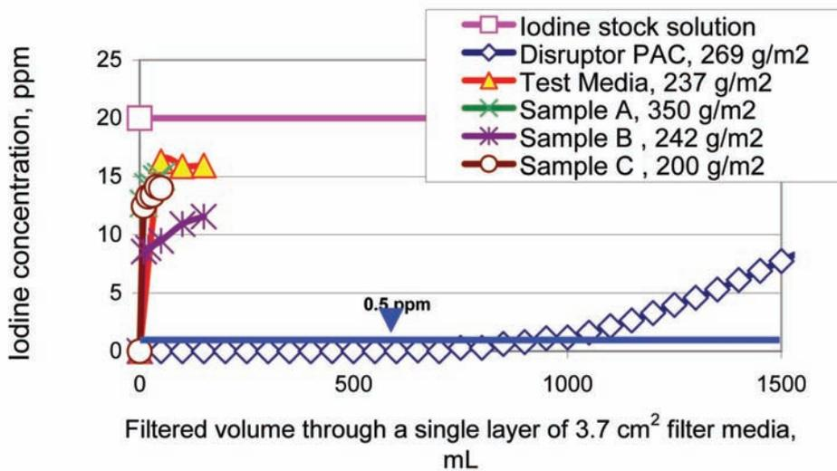
Figure 5 – Iodine Breakthrough Curves for Various Media
