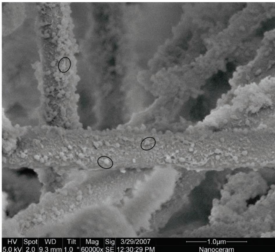
Figure 7: T4-Phages are seen attached to the Disruptor™ fiber. For preparation of the raster electron microscopy (REM) image the filter material was placed for 4 h in a highly concentrated T4-phage solution and dried afterwards. Three phages are encircled as examples, where the icosahedral head and the tail are easily visible
