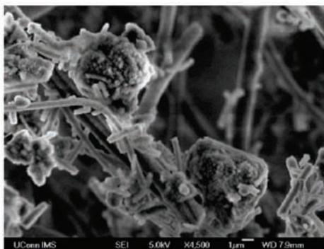
Figure 4 – Powdered Activated Carbon in Disruptor. Photograph by R.Ristau, IMS, UCONN
