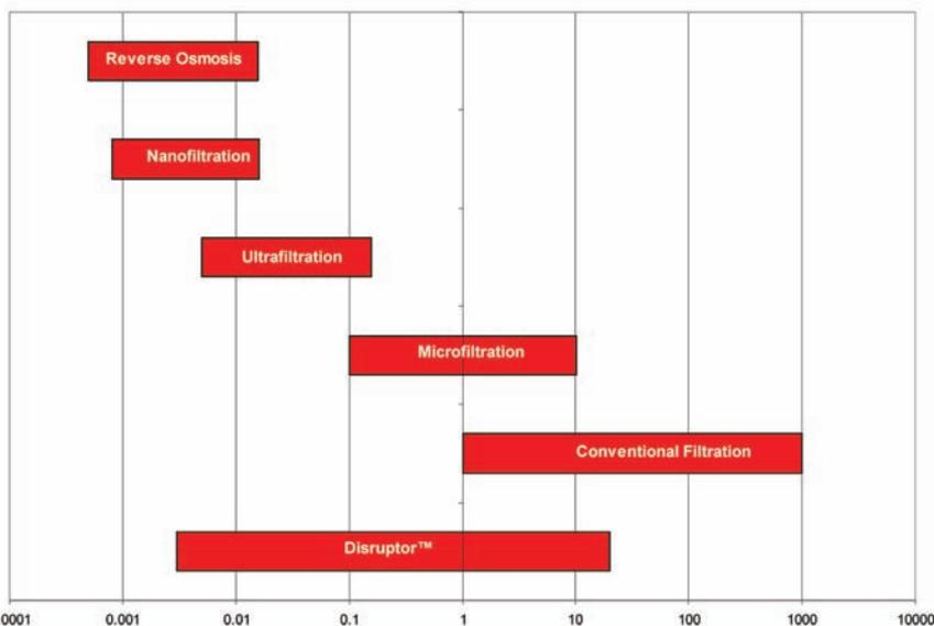
Figure 3- Filtration Spectrum of Disruptor
