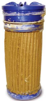
Figure 4. Spent pleated cartridge filter
