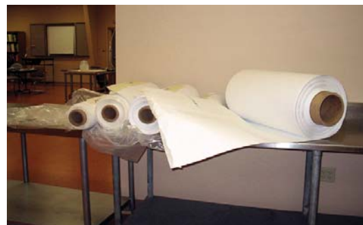
Figure 3. Nano alumina/microglass fiber/cellulose medium
